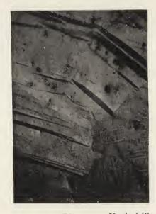
Fig. 14. (x 30 Diameters. Vertical Illumination.) Another view of Fig. 13 after straining.
